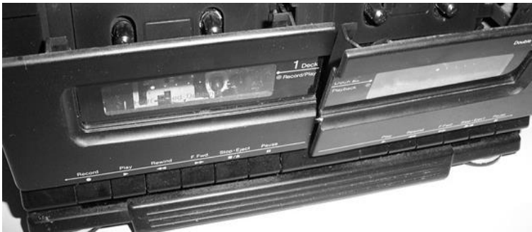
Figure 6 Two cassette lids open at different pace
