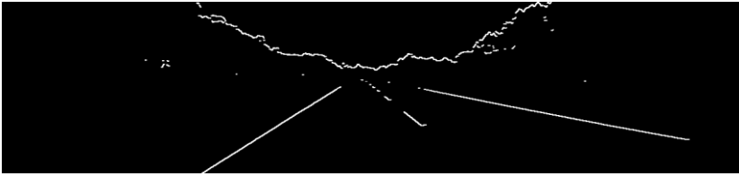
Figure 4. Horizontal Sobel operator.
