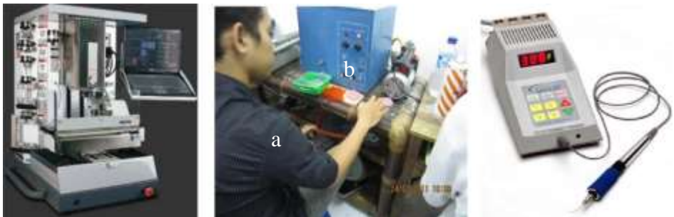
Rajah 4: Mesin Revo 540C (a), Mesin Digital Vacuum Wax Injector (b) dan Mesin Ultra Waxer (c)
