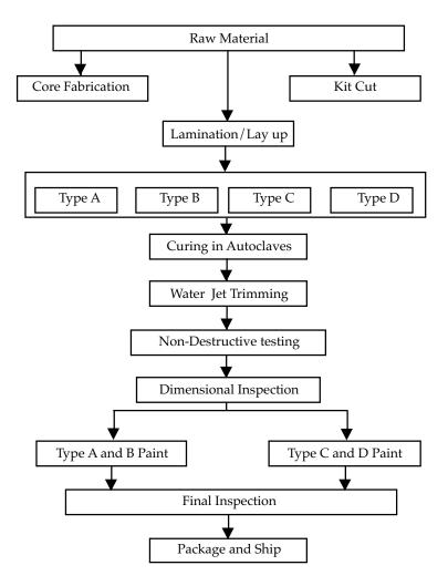
**Figure 2** Schematic of production flows
