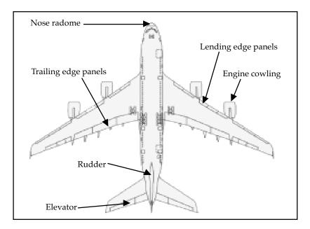
**Figure 1** Plan view of a typical aircraft body.
